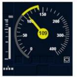
Figure 21 - Speed and supervision information in TSM / ind8 (bubble 1d)
